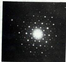
Fig. 2 5–3–2 Fold symmetry of electron diffraction patterns of \text{Al}_{77.5}\text{Mn}_{22.5} bulk sample
