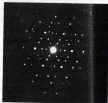
Fig. 2 5–3–2 Fold symmetry of electron diffraction patterns of \text{Al}_{77.5}\text{Mn}_{22.5} bulk sample
