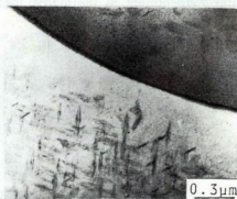
Fig. 4 S' precipitation free zones in grain boundaries
