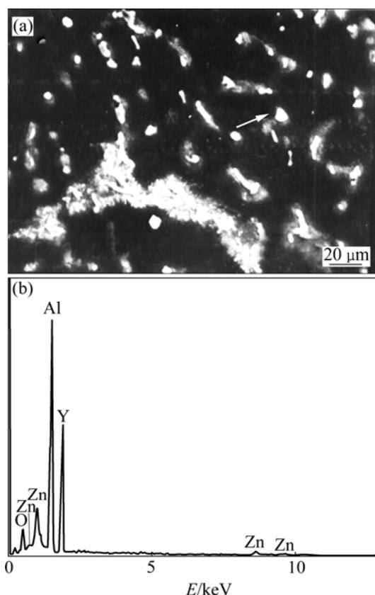
**Fig.4** SEM microstructure (a) and EDX analysis result of secondary phase in alloy 6
