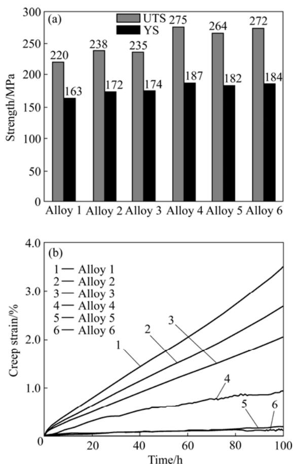
**Fig.2** Tensile mechanical properties (a) and creep behavior (b) of AZ91 and five selected alloys
