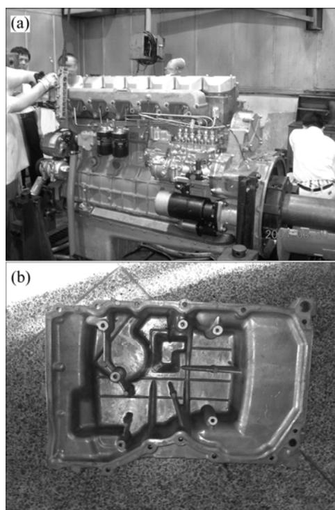
**Fig.5** Application of high temperature creep resistant die-casting Mg alloys: (a) Cylinder head cover; (b) Oil pan
