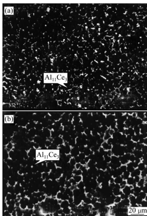
**Fig.3** SEM microstructures of AZ91+0.5Ce alloy before (a) and after (b) creep tests
