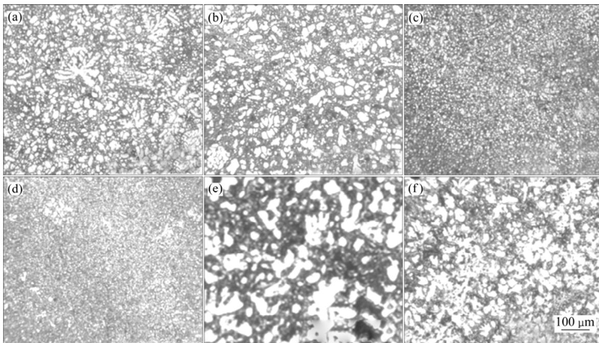
**Fig.1** Microstructures of investigated alloys: (a) Alloy 1; (b) Alloy 2; (c) Alloy 3; (d) Alloy 4; (e) Alloy 5; (f) Alloy 6
