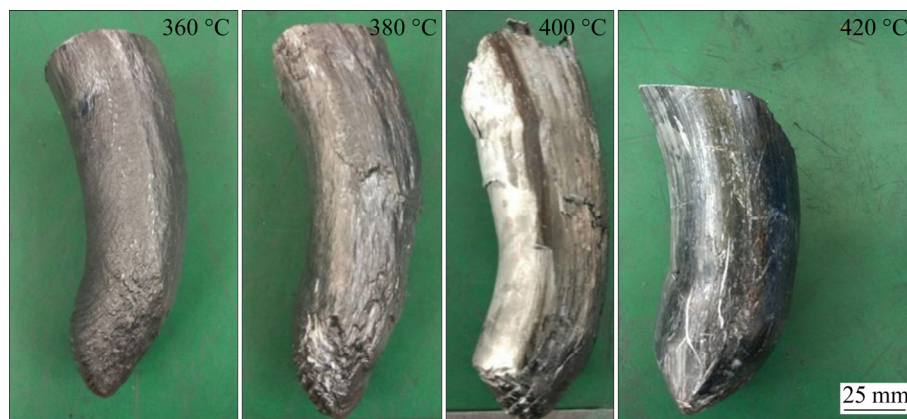
Fig. 8 Macrographs of one-pass ECREed 7005 alloy at different extrusion temperatures
