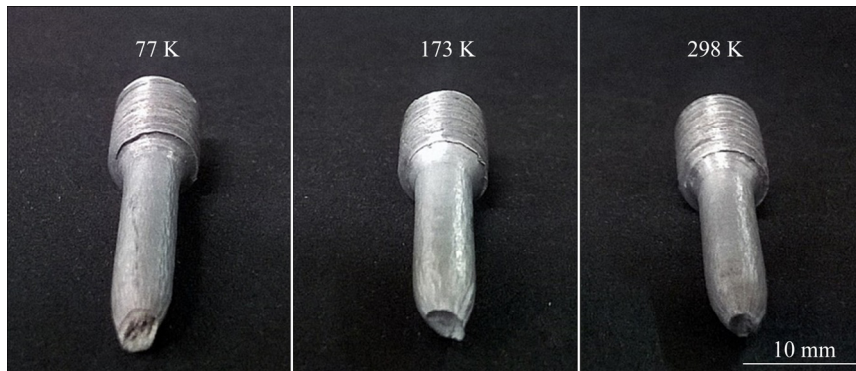
Fig. 6 Photographs illustrating typical fractured specimens of AA6061 alloy after tensile tests at different temperatures showing surface bands in neck region
