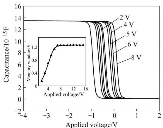
**Fig.2** C-V characteristics of MFIS capacitor with  $\text{CeO}_2$  insulator and BNT ferroelectric layers at various applied voltage (Inset shows corresponding memory window as function of applied voltage)
