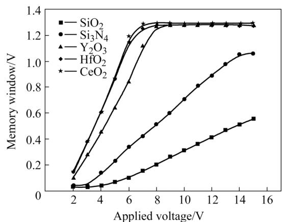
**Fig.5** Memory windows of MFIS capacitors with different insulator layer as function of applied voltage
