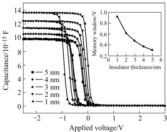
**Fig.3** C-V characteristics of MFIS capacitors with different thicknesses of  $\text{CeO}_2$  insulator layer (Inset shows corresponding memory window as function of insulator thickness)
