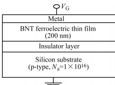
**Fig.1** Schematic illustration of MFIS capacitor structure
