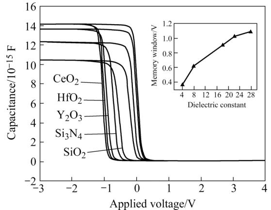
**Fig.4** C-V characteristics of MFIS capacitors with different insulator layers (Inset shows corresponding memory window as function of relative dielectric constant of insulator layer)
