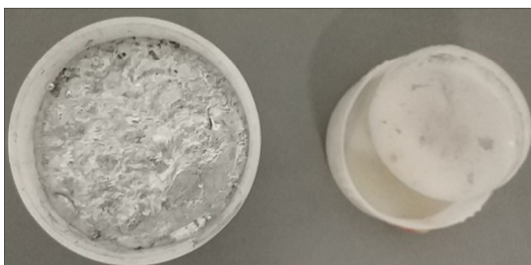
Fig. 2 Raw materials of 4N Ga used in experiment
