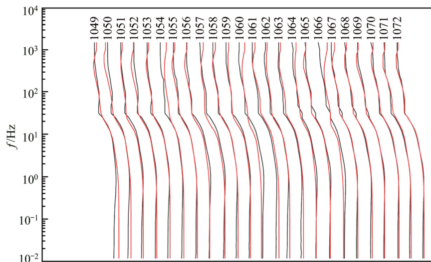
Fig. 14 Apparent resistivity of receivers with source A7B7 after source effect correction (red) and reference curves (black)
