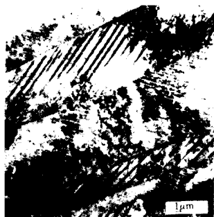
Fig. 5 TEM bright field photography showing twin substructure of B19' martensite
