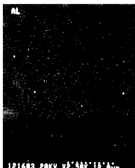
Fig. 4 Al-surface distribution of 5CrMnMo co-diffusion layer
