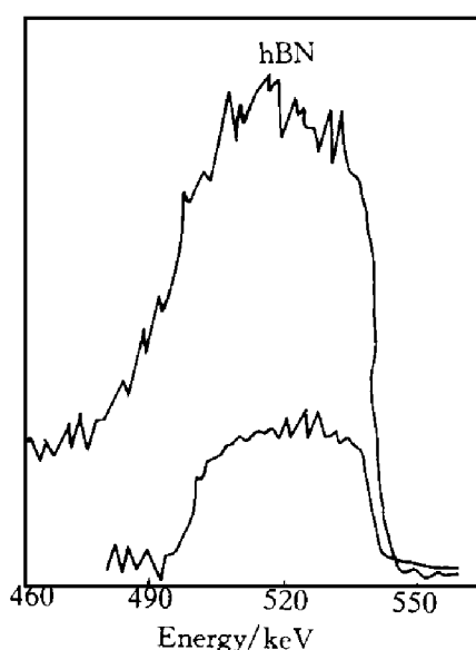
Fig. 3 Nuclear reaction analyses of Ti-B-N film and standard sample (hBN)
