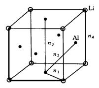
Fig. 1 Al<sub>3</sub>Li crystal structure
