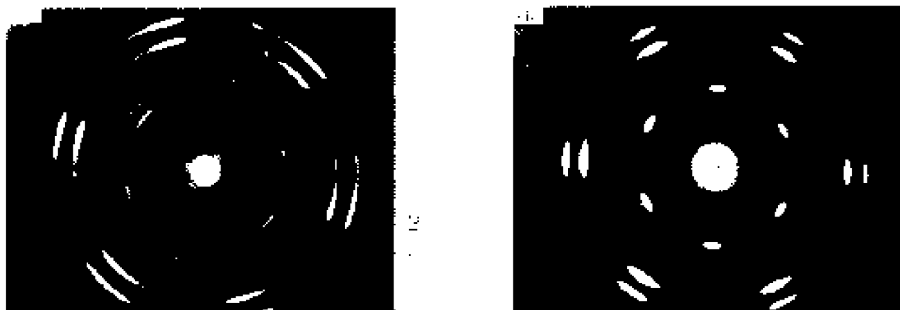
Fig. 1 Selected area electron diffraction patterns of 20/20 (a) and 5/5 (b) multilayered films
