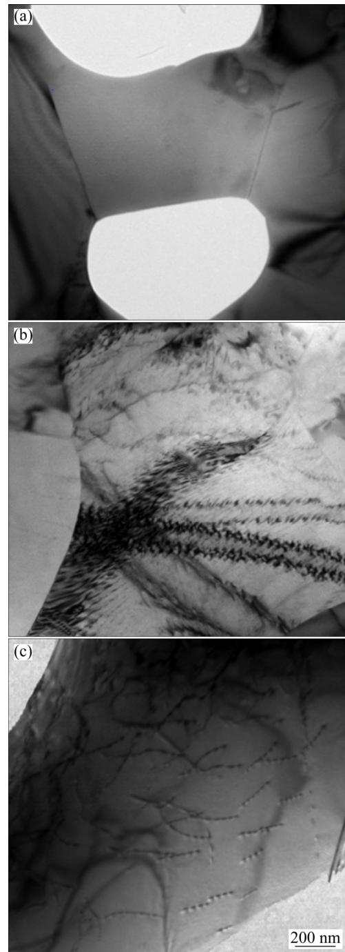
Fig. 9 TEM images after SR testing at 700 °C with different initial grain sizes: (a) 1.25 μm; (b) 4.58 μm; (c) 8.38 μm
