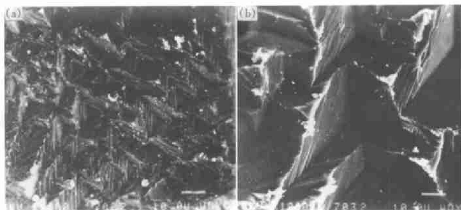
Fig. 2 Surface shapes of uncoated diamond after heated for 10 min in atmosphere (a)—At 900 °C; (b)—At 1050 °C
