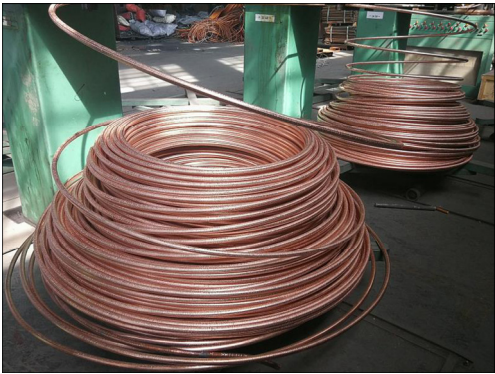
图 15 CuCrZr 合金上引杆坯的宏观照片 Fig. 15 CuCrZr alloy produced by up-drawing continuous casting
