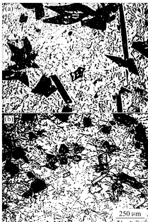
Fig.1 Morphologies of primary silicon in A390 alloy: (a) Un-modified; (b) Modified by 0.1% P for 150 min
