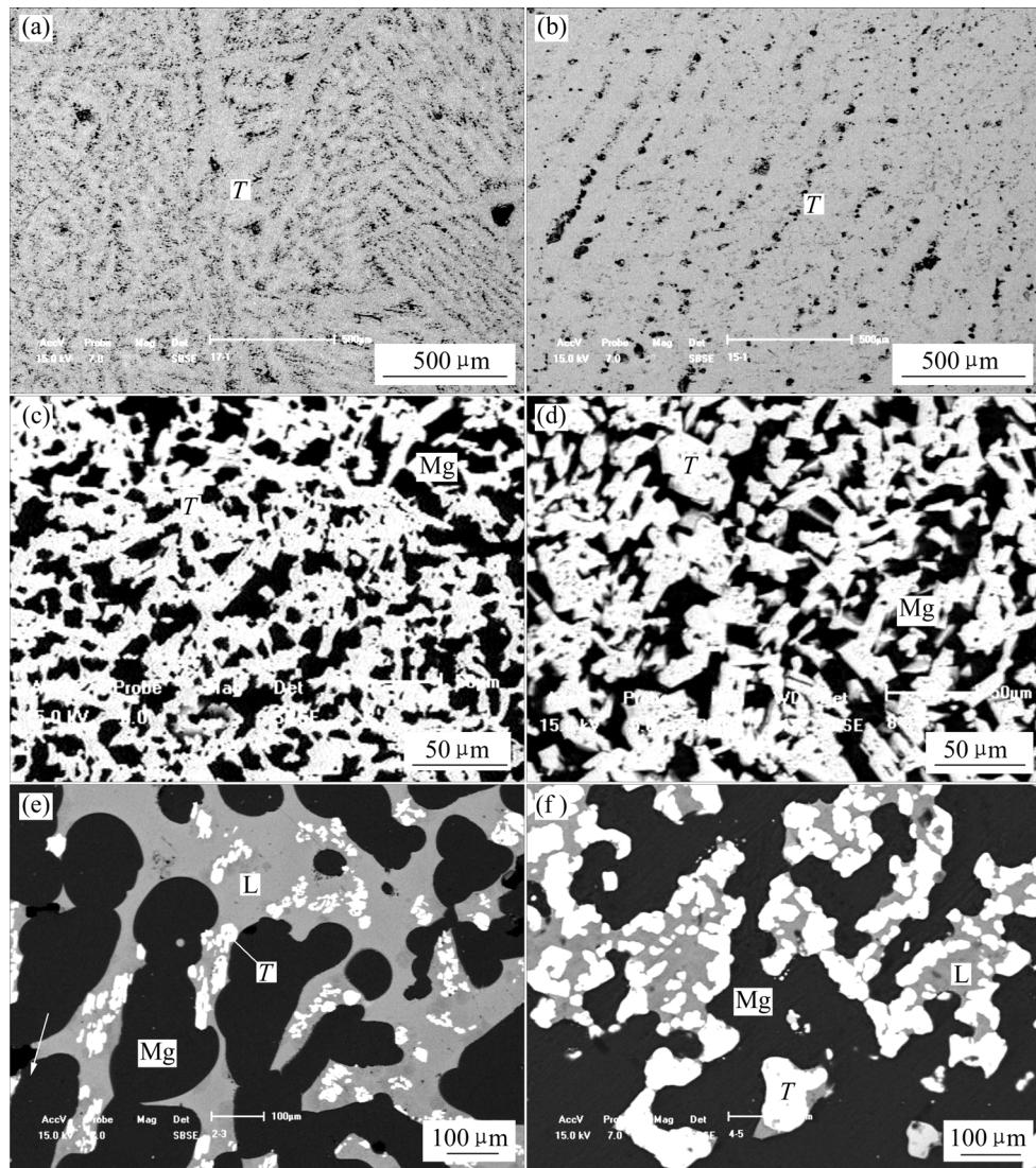
**Fig.2** Equilibrium microstructures of alloys with T-phase at 400 °C (SEM): (a)  $Mg_{67}Zn_{25}La_8$  alloy; (b)  $Mg_{46}Zn_{45.5}La_{8.5}$  alloy; (c)  $Mg_{85}Zn_{10}La_5$  alloy; (d)  $Mg_{80}Zn_{15}La_5$  alloy; (e)  $Mg_{84}Zn_{15}La_1$  alloy; (f)  $Mg_{83}Zn_{15}La_2$  alloy
