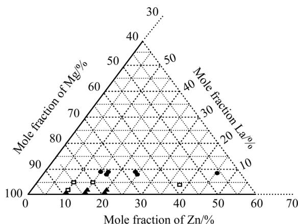
**Fig.1** Compositions of Mg-Zn-La alloys at 400 °C (● Single phase sample; □ Two-phase samples; ▲ Three-phase samples)
