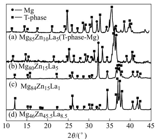
**Fig.4** Comparison of T-phase XRD pattern in different alloys at 400 °C
