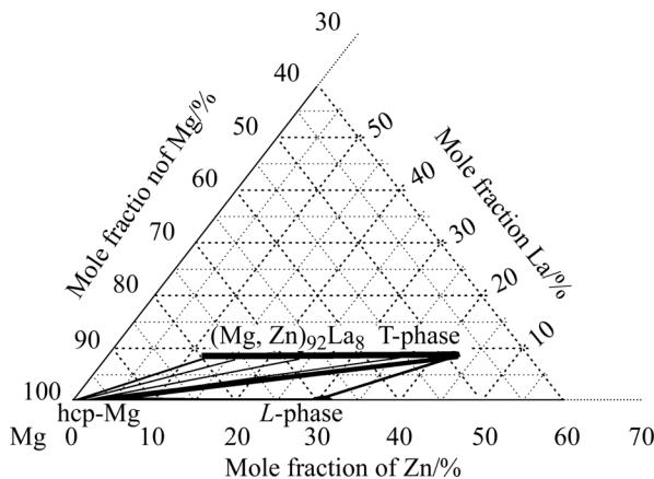
**Fig.5** Isothermal section of Mg-Zn-La system in Mg-rich corner at 400 °C
