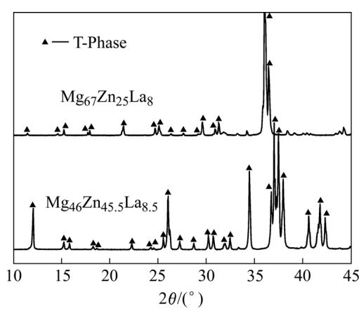
**Fig.3** XRD patterns of single T-phase alloys at 400 °C
