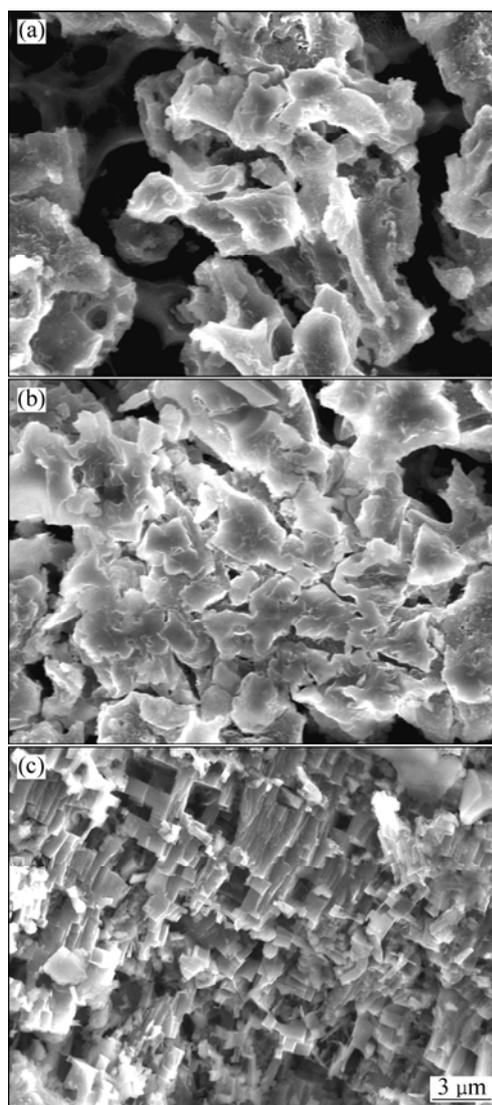
Fig.2 SEM images of cathode surface at different current densities: (a) 5  $\text{mA}/\text{cm}^2$ ; (b) 10  $\text{mA}/\text{cm}^2$ ; (c) 15  $\text{mA}/\text{cm}^2$
