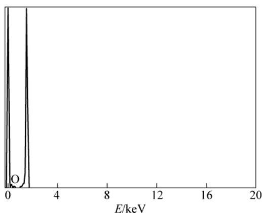
Fig.3 Energy spectrum of cathode surface
