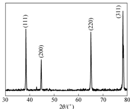
Fig.4 XRD pattern of cathode surface
