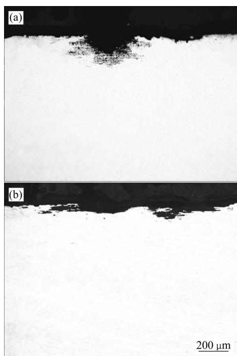
图 4 不同初始状态 2195 铝锂合金蠕变峰值时效晶间腐蚀 Fig. 4 Intergranular corrosion of peak creep aging for 2195 Al-Li alloy under different initial conditions: (a) CA1 specimen; (b) CA2 specimen
