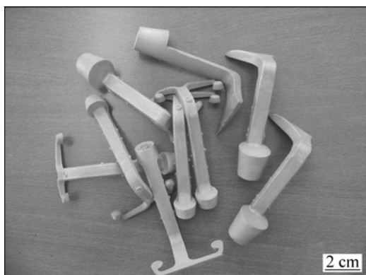
Fig.1 AZ91D magnesium alloy scraps produced in die casting
