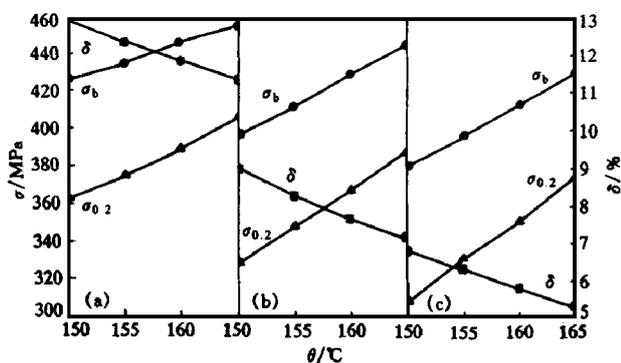
Fig.3 Mechanical properties of 2014 alloy forgings versus aging temperature (a) — Along LD; (b) — Along TD; (c) — Along HD
