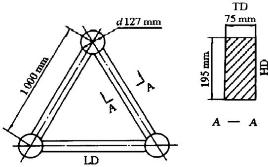
Fig. 1 Shape and dimension of studied forgings
