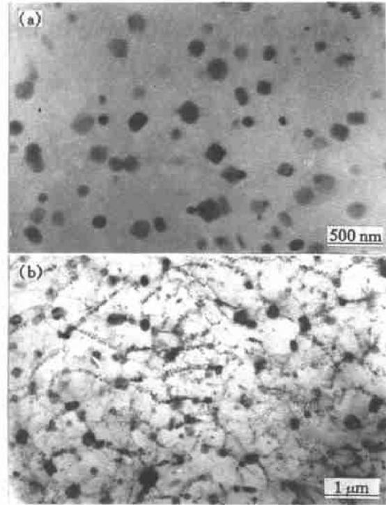
Fig. 2 TEM images of forgings with different deformation coefficients and solutioned at 500 °C for different times
