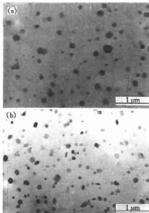
Fig.4 TEM images of forgings at different aging temperatures (a) —150 °C ; (b) —165 °C
