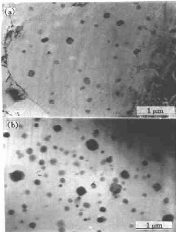
**Fig.7** TEM images of aged forgings by traditional process
