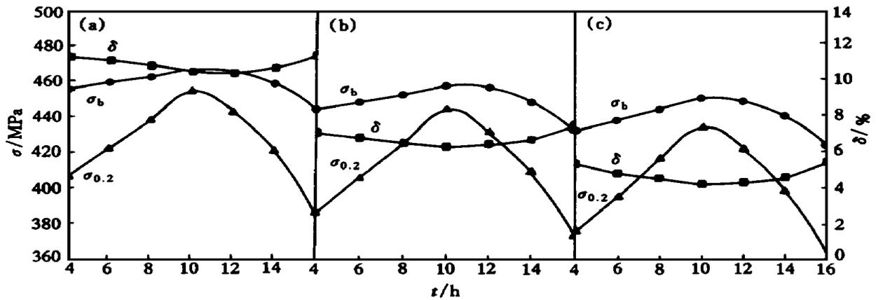
**Fig.5** Mechanical properties of 2014 alloy forgings versus aging time
