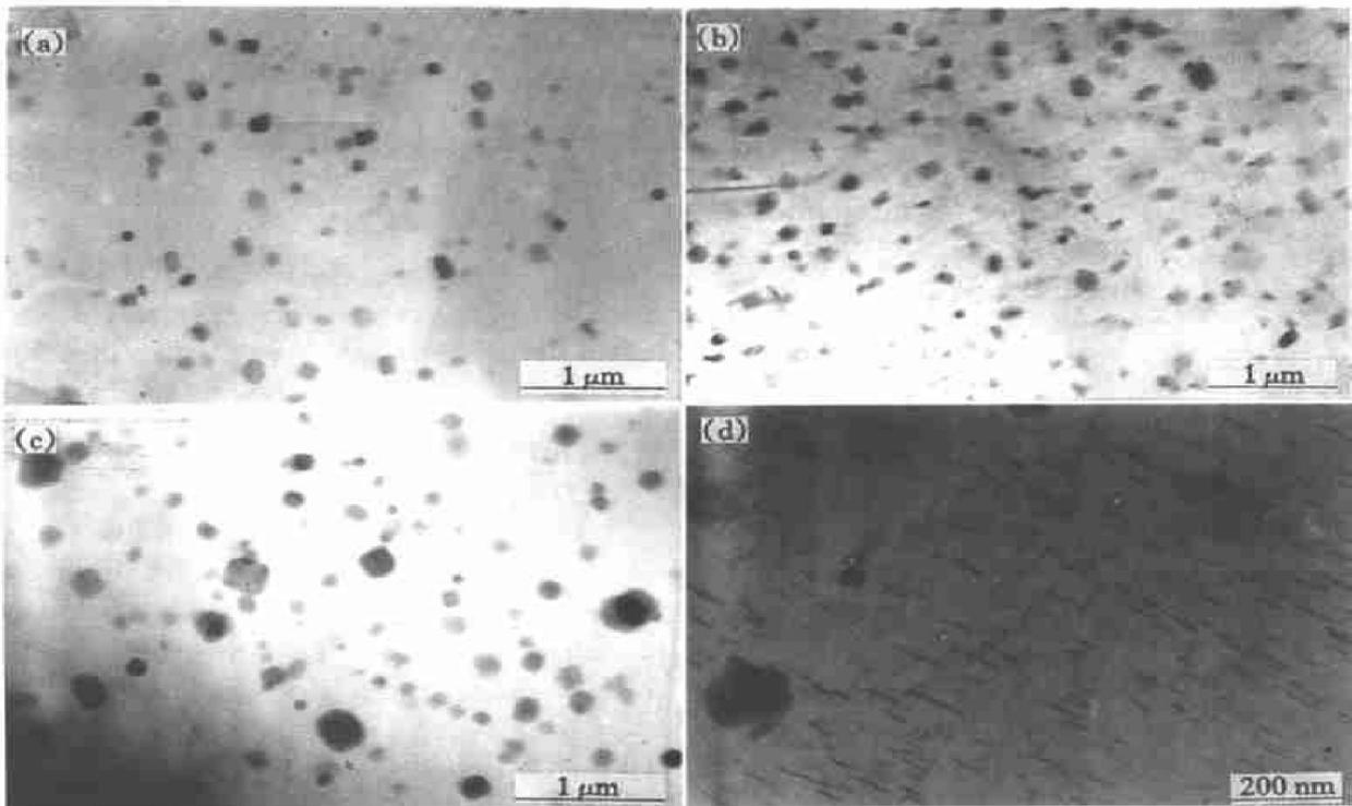
**Fig.6** TEM images of forgings aged at 165 °C for different times
