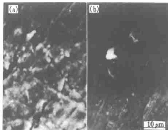
Fig. 4 Micro-fissures and arc craters on surfaces of tantalum oxides
