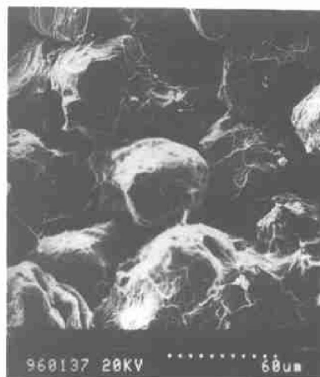
Fig.3 SEM micrograph of fracture surface of tensile specimen
