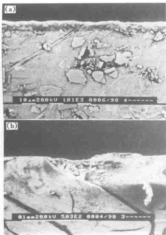
Fig.6 Cross section images of PRAMC and friction surface of cast iron in braking (a) —PRAMC; (b) —Cast iron
