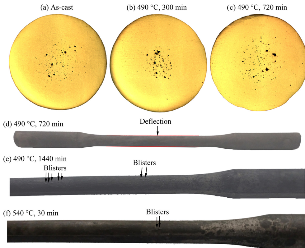
Fig. 2 Sections (a–c) and appearance (d–f) of tensile bars
