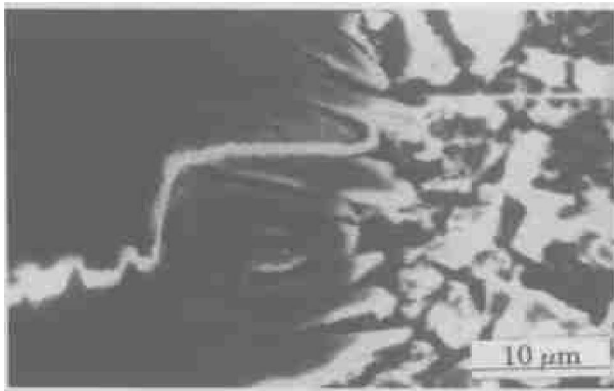
Fig.5 Fe K_{\alpha} line scan
