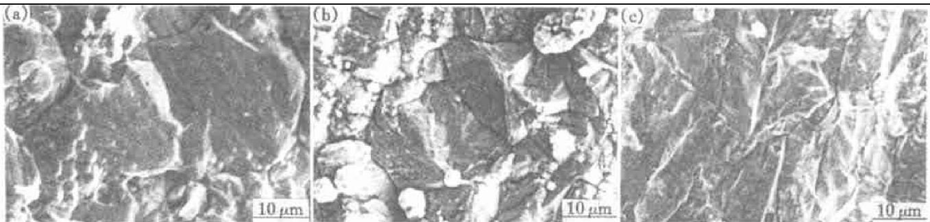
Fig. 9 Corrosion morphologies of Cu-Ni alloy tubes immersed in natural seawater for 48 months (a) —Specimen H; (b) —Specimen A
