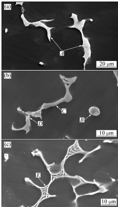
**Fig.4** SEM images of as-cast alloys: (a) ZA62; (b) ZAX6205; (c) ZAX6210
