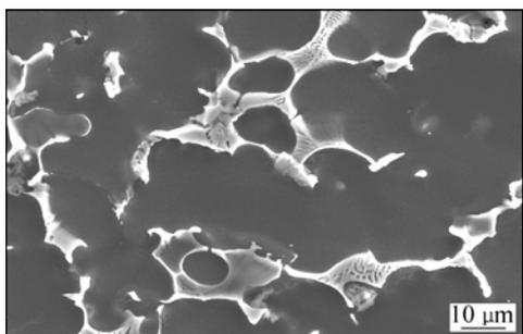
**Fig.8** Microstructure of alloy ZAX6210 after creep at 175 °C, 70 MPa for 100 h
