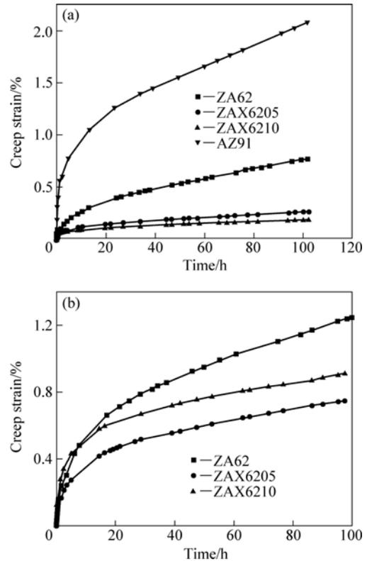
**Fig.7** Creep curves of experimental alloys for 100 h: (a) At 150 °C, 70 MPa; (b) At 175 °C, 70 MPa**Table 4** Steady creep rate and 100 h creep strain of different alloys at 70 MPa
