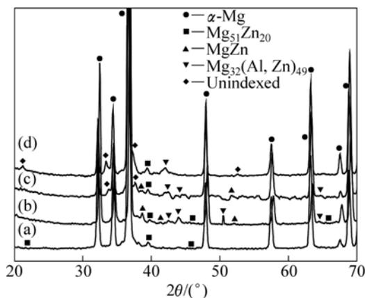
**Fig.3** XRD patterns of as-cast alloys: (a) ZA62; (b) ZAX6202; (c) ZAX6205; (d) ZAX6210
