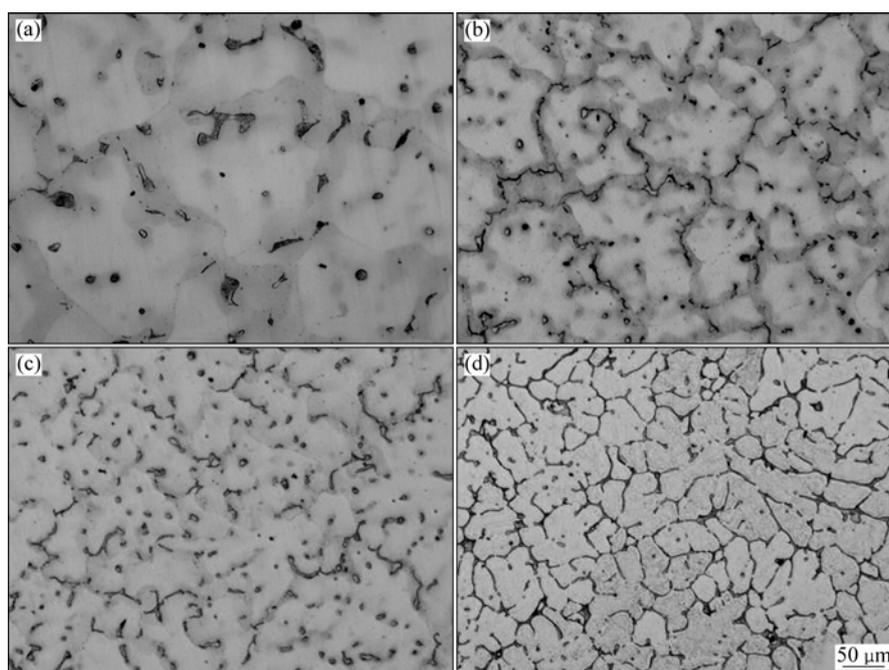
**Fig.1** Optical micrographs of as-cast alloys: (a) ZA62; (b) ZAX6202; (c) ZAX6205; (d) ZAX6210
