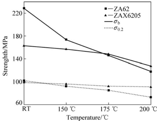
**Fig.6** Tensile properties of alloys at different temperature
