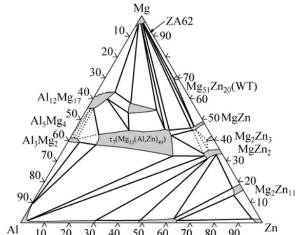
**Fig.5** Isothermal section of Mg-Zn-Al ternary diagram at 335 °C
