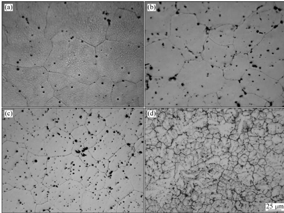
**Fig.2** Optical micrographs of alloys after annealing treatment at 340 °C for 120 h: (a) ZA62; (b) ZAX6202; (c) ZAX6205; (d) ZAX6210
