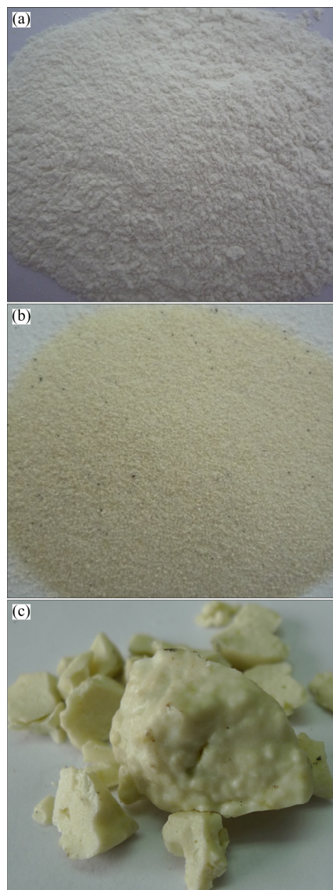
Fig. 1 Macrostructures of calcium aluminate clinkers with different P additions: (a) Without P; (b) 0.50% P; (c) 0.85% P
