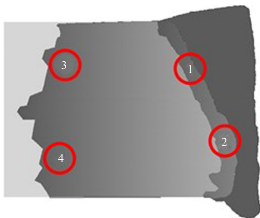
Fig. 3 Section for TEM analysis in HAZ of welded joints
