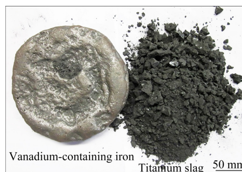
Fig. 11 Macro picture of vanadium-containing iron and titanium slag
