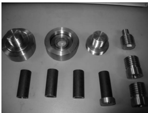
Fig.1 16 mm-diameter steel tubular model specimens and chucks
