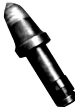
**Fig.1** Cutting pick strengthened by plasma jet surface metallurgy
