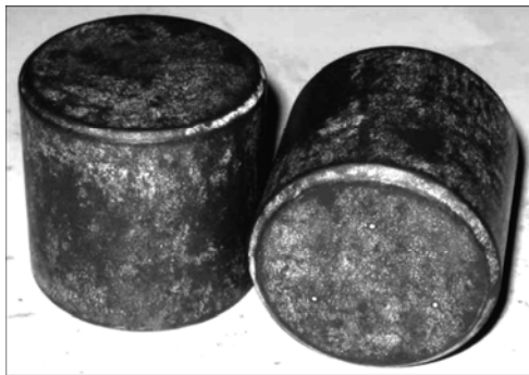
Fig.1 Workpiece after phosphate coating and soaping process
