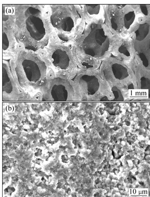
**Fig. 1** Morphologies of SiC foam reinforcement: (a) Macro-appearance; (b) Surface of strut
