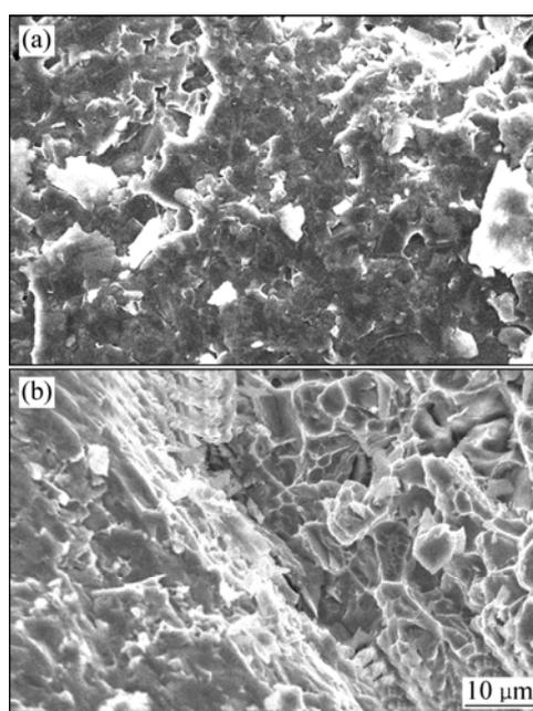
**Fig.4** Fractographs of SiC foam-SiC particles/Al hybrid composites: (a) Foam strut; (b) Interface
