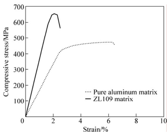
**Fig.3** Relationship between stress and strain for composites reinforced by different matrix
