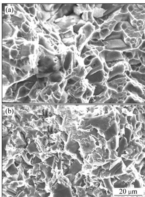
**Fig.5** Fractographs of SiC particle and matrix in composites with different matrix: (a) Pure aluminum; (b) Aluminum silicon alloy ZL109
