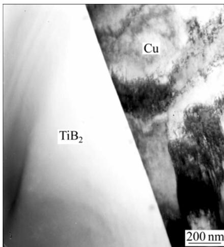
Fig.4 TEM micrographs of TiB<sub>2</sub>-Cu interfaces
