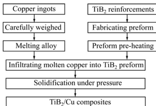
**Fig.1** Flow chart of squeeze casting technology used for fabricating  $\text{TiB}_2/\text{Cu}$  composites
