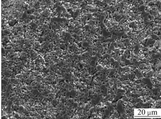
Fig.3 Microstructure of TiB<sub>2p</sub>/Cu composite
