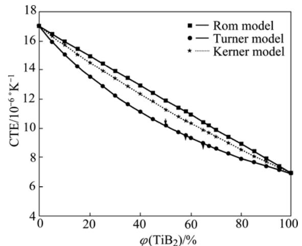
Fig.5 Comparison between theoretical predictions and experimental CTEs
