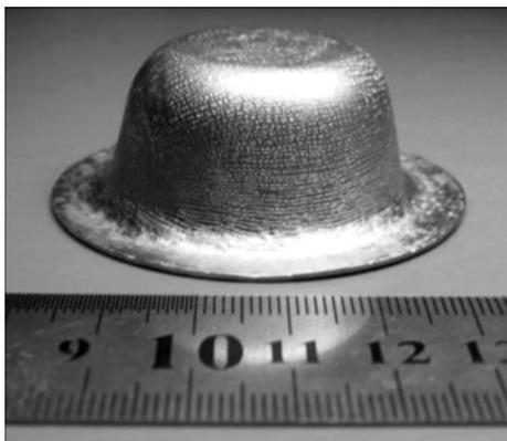
**Fig.11** Ti6Al4V deep cylinder superplastically formed by ceramic die
