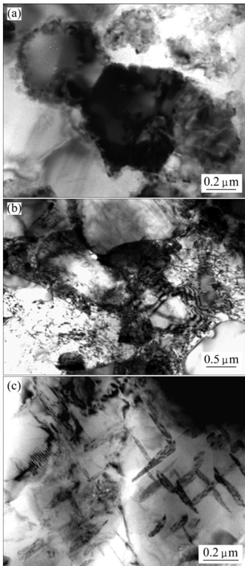
**Fig.3** TEM images of as-cast and extruded  $\text{Si}_3\text{N}_4\text{p}/2024\text{Al}$  composite: (a) As-cast composite; (b) Extruded composite; (c) Extrusion and T6 treated composite
