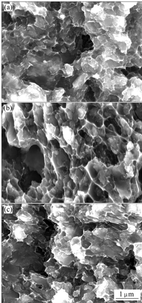
**Fig.6** Tensile fractured surface morphologies of composite: (a) As-cast composite; (b) T6 treated composite; (c) Extrusion and T6 treated composite
