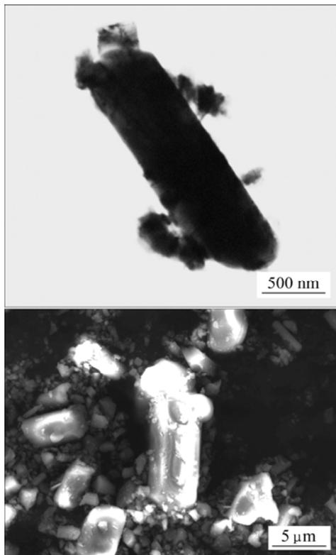
**Fig.1** Morphologies of  $\text{Si}_3\text{N}_4$  ceramic particles
