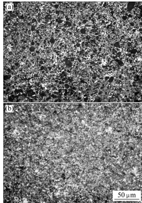
**Fig.2** Microstructures of as-cast and extrusion  $\text{Si}_3\text{N}_4$ /2024Al composite: (a) As-cast composite; (b) Extruded composite
