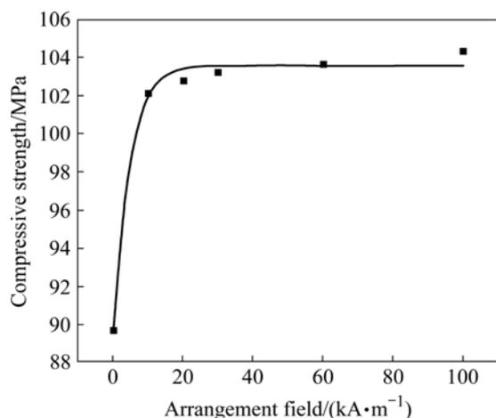
**Fig.11** Relationship between compressive strength and arrangement field
