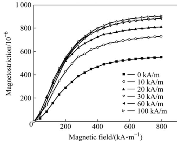
Fig.4 Relationship between static magnetostriction and applied field for specimen prepared under different arrangement fields
