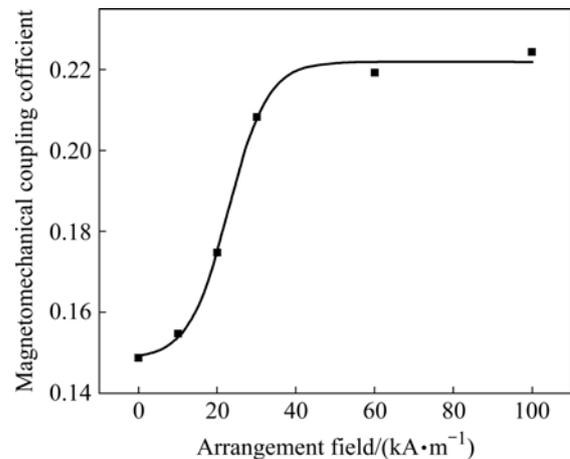
**Fig.9** Relationship between magnetomechanical coupling coefficient and arrangement field at 42 kA/m bias field
