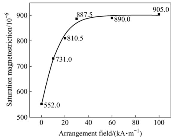
Fig.5 Relationship between saturation magnetostriction and arrangement field
