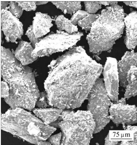
Fig.1 Irregular shape of Terfenol-D particles
