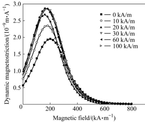
**Fig.6** Relationship between dynamic magnetostriction and applied field
