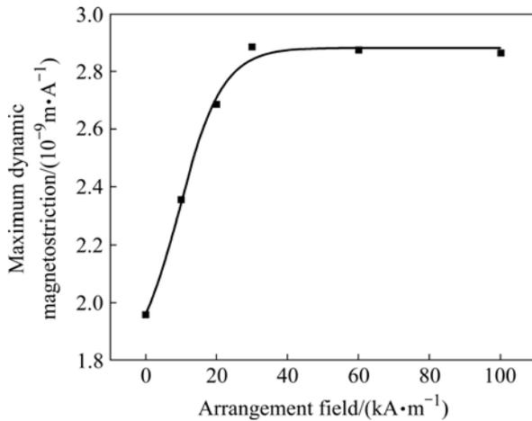
**Fig.7** Relationship between maximum dynamic magnetostriction and arrangement field
