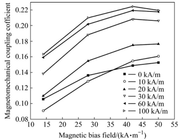
**Fig.8** Relationship between magnetomechanical coupling coefficient and magnetic bias field
