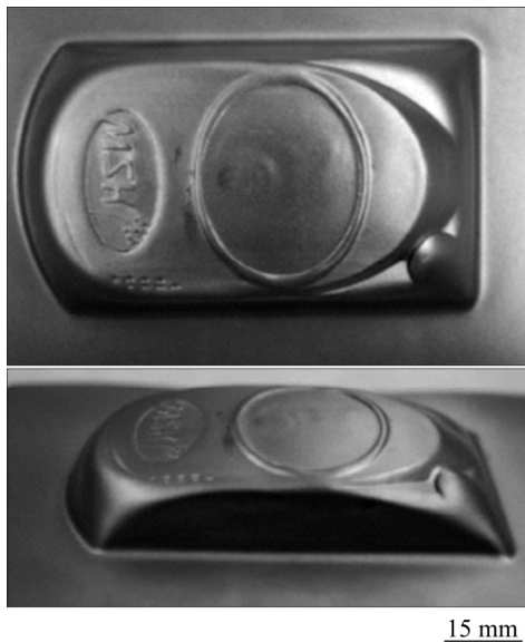
Fig. 1 CP titanium sheet formed by hybrid forming technique at input energy of 6.4 kJ
