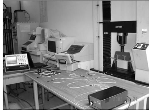
Fig.9 Experimental setup of four-point bending measured by Mach-Zehnder interferometry
