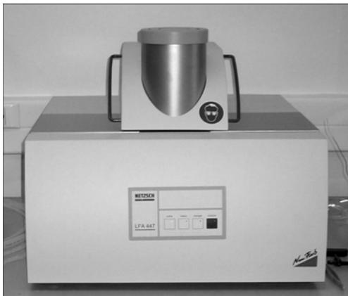
Fig.1 Thermal conductivity test equipment (LFA447)
