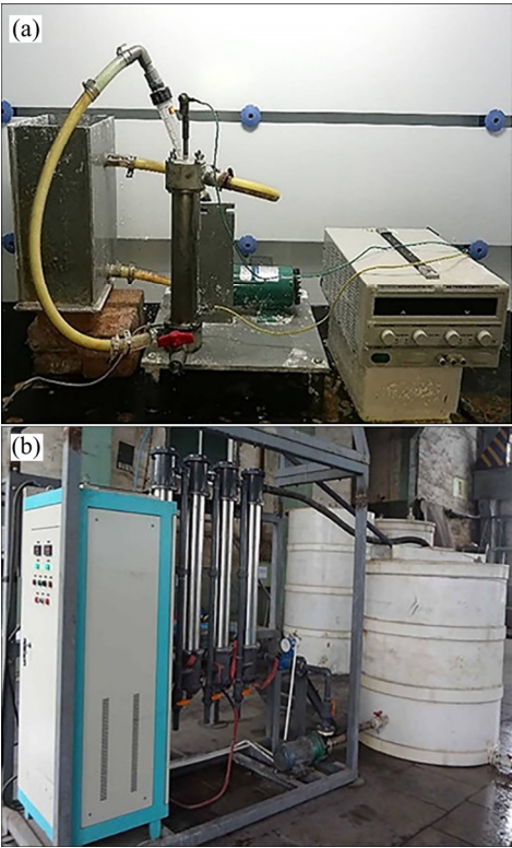
图 1 旋流电积槽 Fig. 1 Pictures of cyclone electrowinning cell: (a) Laboratory-scale reaction devices; (b) Pilot plant
