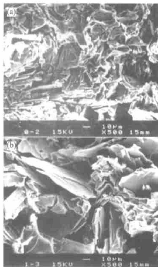
Fig. 6 SEM microstructures of Al-7% Si alloy (a) —Without EMS; (b) —Solidified with EMS at 170 V
