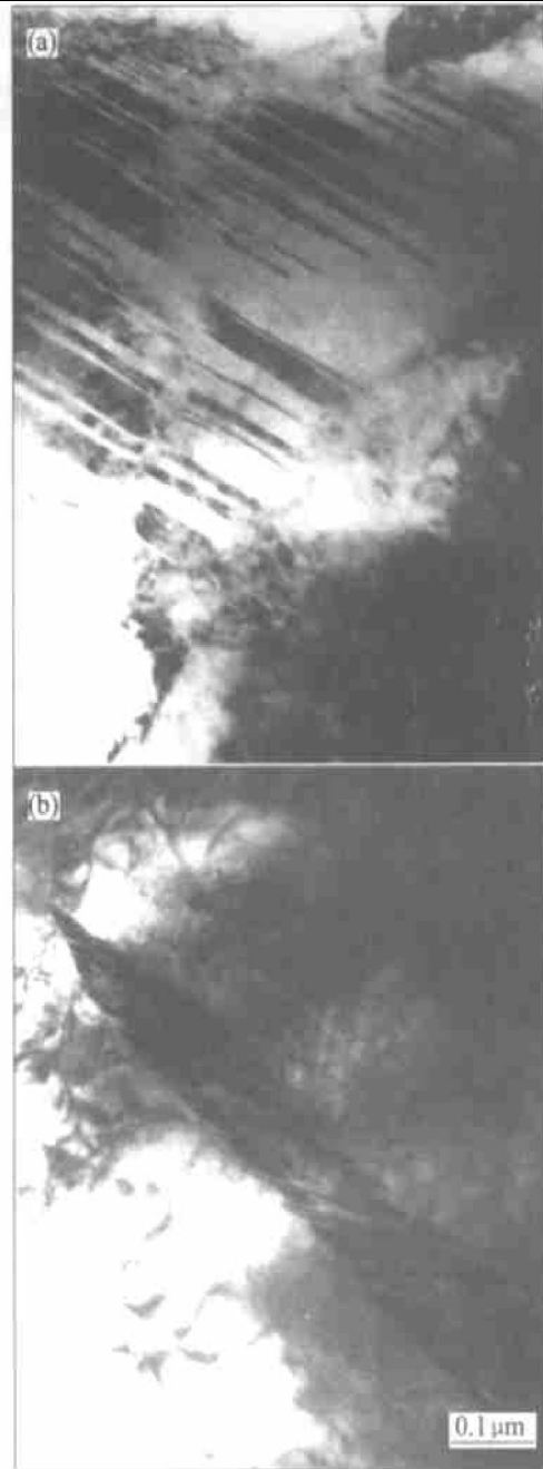
Fig. 12 TEM images of ZrO_2(2Y)/TRIP steel composites under dynamic load (a) —TZ20; (b) —TZ25
