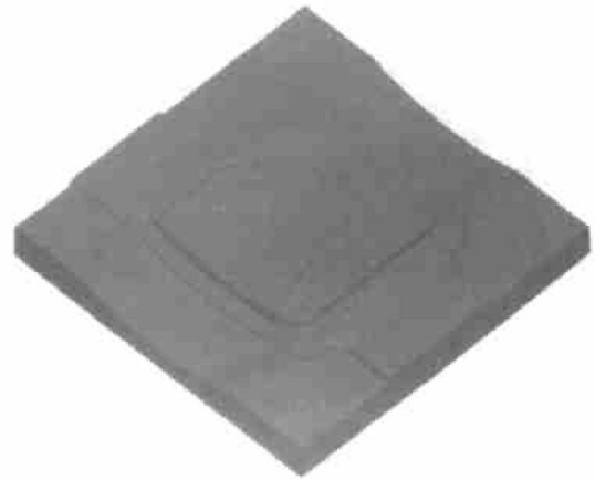
Fig. 5 Second-step drawing CAD model of die
