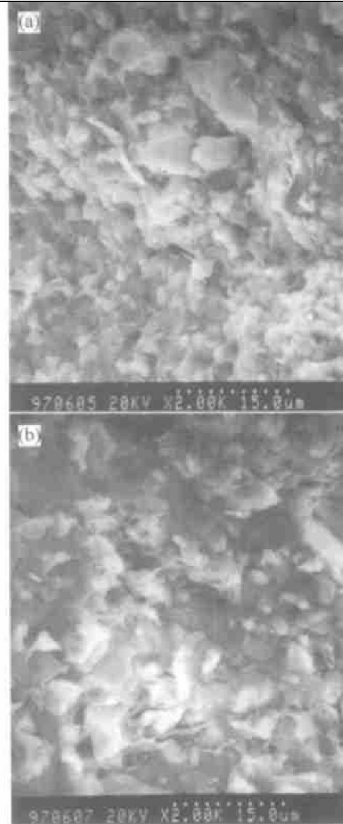
Fig. 4 SEM micrographs of fracture surfaces of composites (a) —BT20; (b) —BT30
