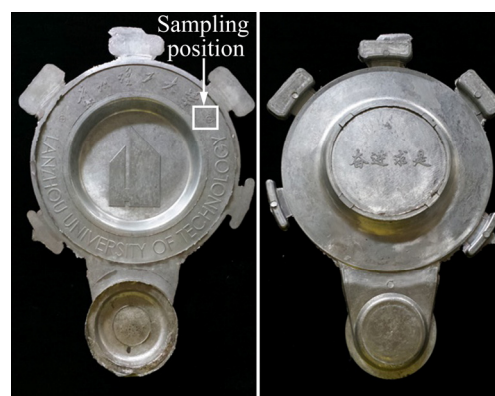
Fig. 2 Die casting component and sampling position
