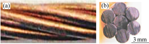
图 2 铜绞线宏观照片 Fig. 2 Photos of copper stranded wire: (a) Longitudinal direction; (b) Cross section
